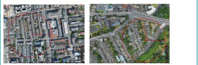
Figure #8-2: Examples of using satellite view (Google) to help score this question: these two sites in East London have similar built typologies with mostly low-rise housing and some isolated high-rise blocks, and would score the same for overall urban heat island effect (#2) because of their location in Tower Hamlets and Hackney. However, at the local scale (100m radius) they have very different characteristics in terms of green infrastructure, with the left-hand side site likely to experience higher local temperatures.
